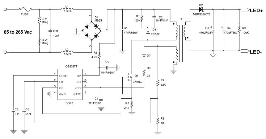
Figure 6: OZ8027T Typical Application Schematic
