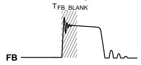
Figure 4: Ringing waveform of FB voltage
